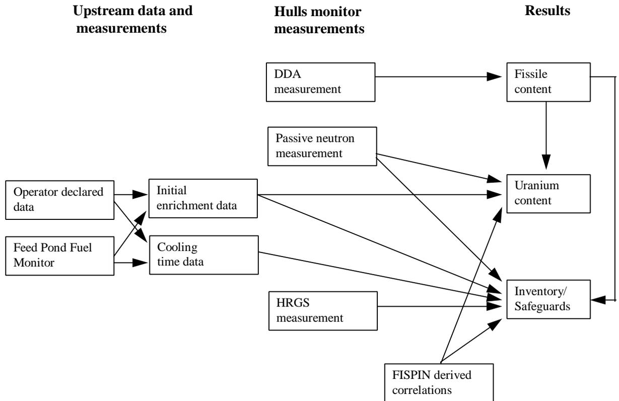
Fig. 2 Information Flow in the THORP Hulls Monitor
