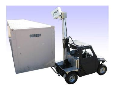
"A fully integrated utility vehicle for nuclear materials detection and measurement"
